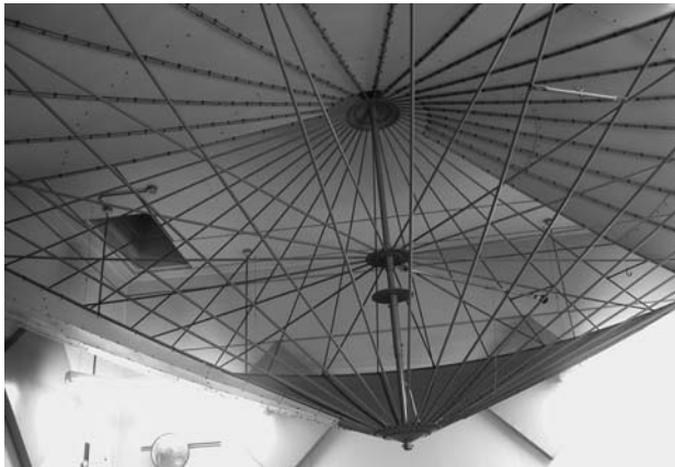
The Indianapolis engineering facility includes a reverberant sound room with rotating vane to test sound ratings of HVAC equipment.
