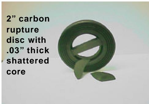
**2" carbon rupture disc with .03" thick shattered core**
